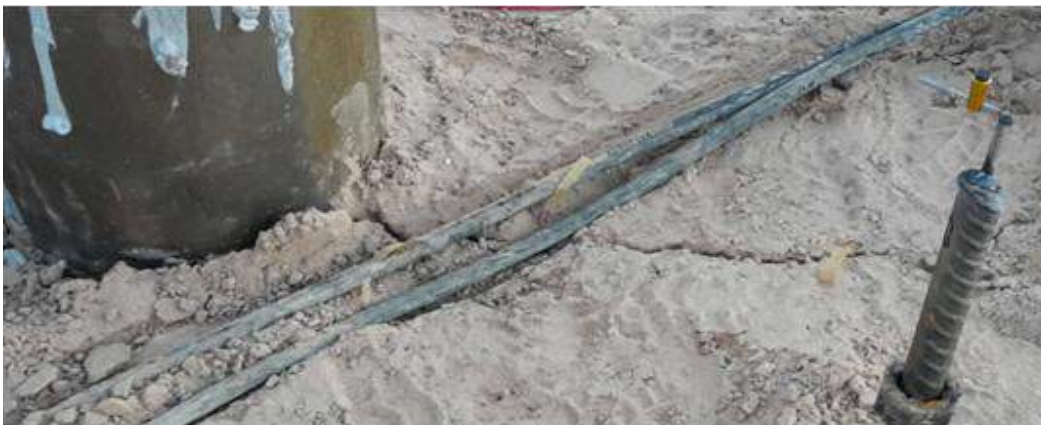
Fig. 16b Photographs of cracks in ground surface stretching from one pile toward the next along the side of the group.
